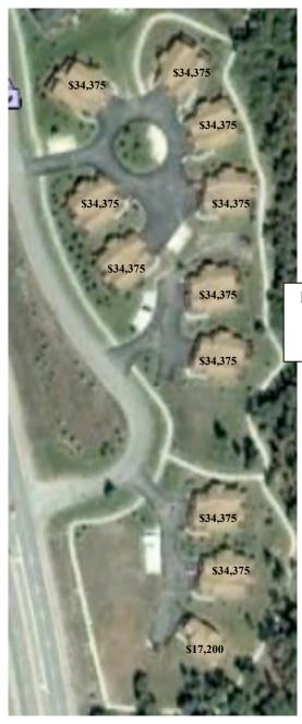
Higher relative cost for duplexes due to more complicated roofline and required flat roof material at cricket sections between each duplex.
