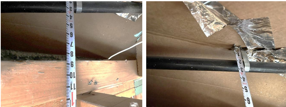
Figure 12. Measurements for the high point of the cardboard and distance of pipe from the cardboard (16020_CBS_2-054, 16020_CBS_2-055).
