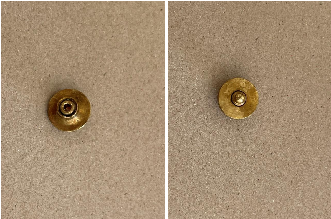
Figure 22. Component of the sprinkler seat/plug (16020_CBS_2-031, 16020_CBS_2-032).
