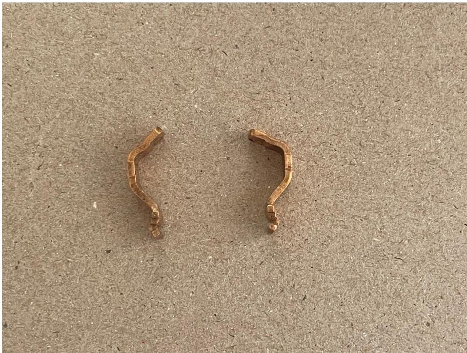
Figure 23. Tension arms from the subject sprinkler (16020_CBS_2-035).
