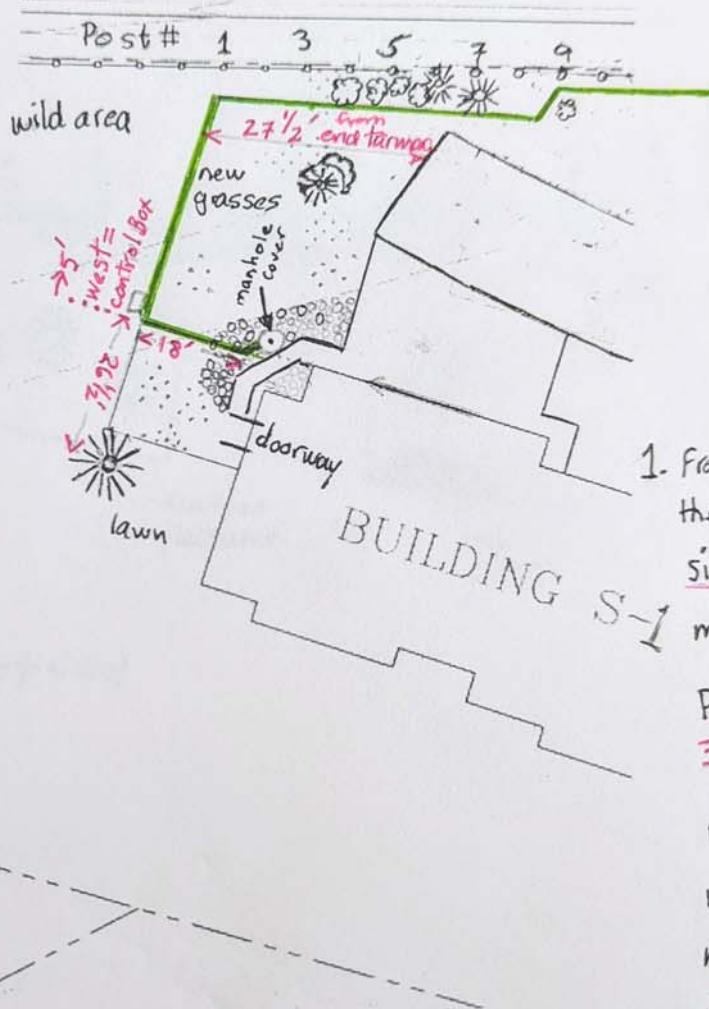
1. From the front wall of Bldg S-1, the manhole cover touches the sight-line looking south. The main irrigation line runs south; parallel to the sight-line. 3' east of the ⚭ of the manhole cover - for 18' where it turns west. A new control box is located 5' west of this  $90^\circ$  bend.
